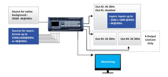
Use case 4: 4K LiveCore<sup>™</sup> with two 4K 30Hz 4:4:4 outputs
