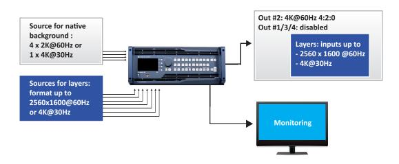
In this configuration, output #2 generates a 4K 60Hz 4:2:0 format. All the other outputs are disabled.
