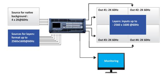
In this configuration, four 2K 60Hz outputs (3G-SDI or DVI) are used in hard-edge mode to create a 4K screen. The native background is composed of four unscaled 2K 60Hz inputs or four 2K still frames, each assigned to an output.
