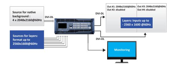
In this configuration, two DVI Dual-Link outputs (2048x2160) are used side by side in hard-edge mode to create a 4K screen. The native background is composed of two unscaled 2048x2106@60Hz DVI Dual-Link inputs or two 2048x2160 still frames, each assigned to an output.
