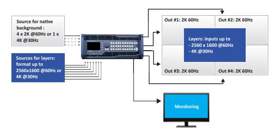
In this configuration, four 2K 60Hz outputs (3G-SDI or DVI) are used in hard-edge mode to create a 4K screen.
