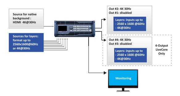
In these configurations, at least one of the outputs generates a 4K 30Hz 4:4:4 format. The adjacent output is disabled (the implementation is similar to dual-link output setup). For LiveCore<sup>™</sup> series with four outputs, the remaining outputs can be configured either in 2K (use case 2) or in 4K (use case 3).
